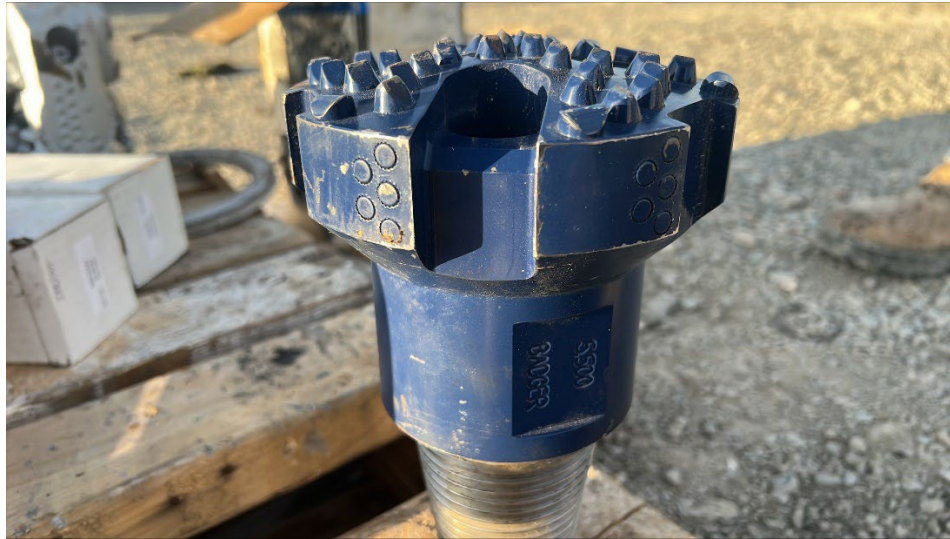
Figure B.3-25. This bit (the Badger) was effective in milling out the customized frac plugs.
