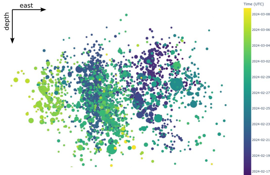
Figure B.5-12. The advanced detection and location workflow qseek clearly shows planar features within the reservoir of Cape Station. The automated event locations shown here only include events above M0.
